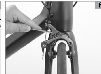
See your SCOTT dealer and ask him to examine the remaining thickness of the rims when you are through your second set of brake pads at the latest. Your SCOTT dealer has special measuring devices for determining the remaining thickness of the rims.
