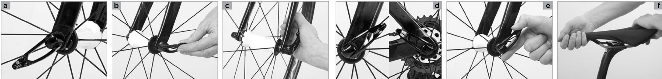
If your seat post is equipped with a quick-release mechanism, check whether the saddle is firmly fixed by trying to twist it relative to the frame **(f)**.
