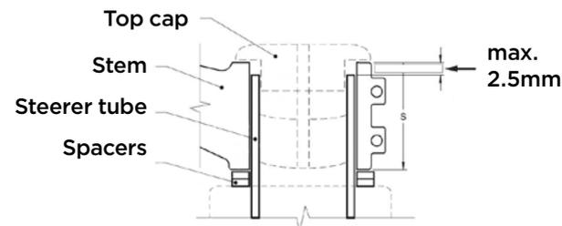
7. Clamp the stem onto the steerer tube with a maximum of 6 Nm (f) and respect also the maximum torque value of the stem manufacturer. The lower value indicated on these components has to be accepted as a maximum torque value. Do not overtighten!
