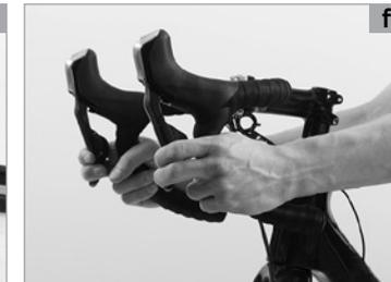
With disc brakes **(a)** you should have a stable pressure point at once. If you have to actuate the brake lever more than once to get a positive braking response, have the SCOTT bike checked by your SCOTT dealer immediately. For more information see the chapter “Brakes” and the manuals of the component manufacturers on this SCOTT info CD.
