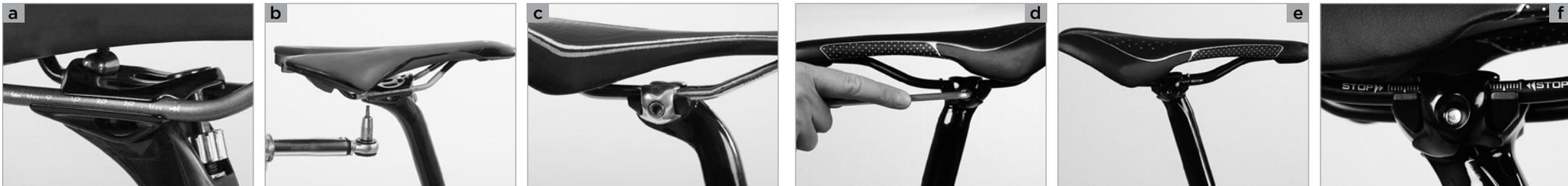
Position the saddle so that its upper surface is parallel to the ground. Tighten the bolt gradually and make sure
