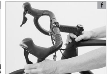
To check whether the headset runs smoothly, lift the frame up until the front wheel no longer touches the ground. The handlebars should turn from far left to far right without feeling roughness or tightness at any point. With a gentle tap on the handlebars the fork should turn easily from the middle position **(a)**.
