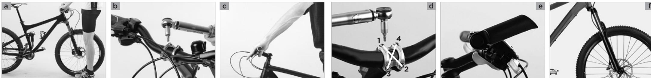
Damping is usually done by oil. To work perfectly, the fork has to be adjusted to the weight of the rider, the sitting posture and the intended use **(a)**. Be sure to have this adjustment carried out by your SCOTT dealer at the time of delivery. For more information see the chapter “Front suspension” in your detailed SCOTT owner’s manual as well as in the manuals of the suspension fork manufacturer on the enclosed SCOTT info CD.
