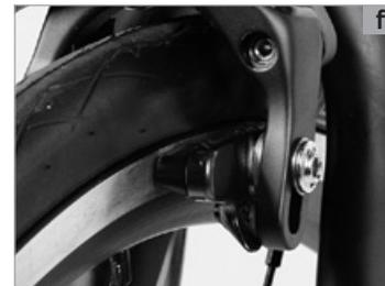
Actuate both brakes simultaneously (e) and bear in mind that, due to the weight transfer, the front brakes can generate a far better braking effect on a surface with good grip.
