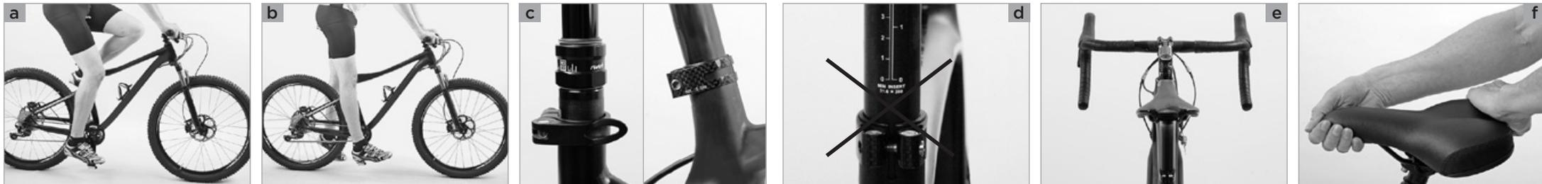
Check whether you can touch the ground safely while sitting on the saddle by stretching your feet to the floor **(a)**. If not, you should lower the saddle until you can, at least to begin with.
