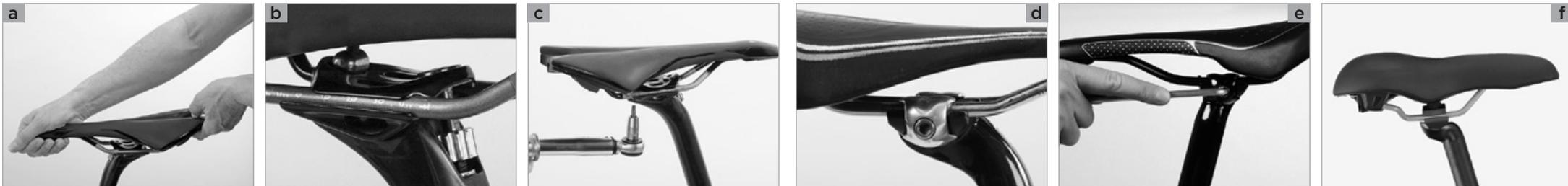
If the saddle rails fit into the clamp grooves, slide the saddle on the seat post and ensure that the clamp is positioned midway along the total length of the rails **(a)**. Position the saddle so that its upper surface is parallel to the ground. Tighten the bolt gradually and make sure
