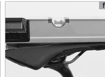
Having found your preferred position, make sure both clamp halves fit snugly around the saddle rails before tightening the bolt(s) to the correct torque value as prescribed by the seat post manufacturer.
