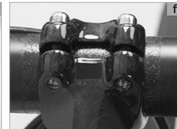
Tighten the bolts evenly and in a cross pattern, i.e. alternately and gradually, to the lower value of the recommended torque values using a torque wrench.
